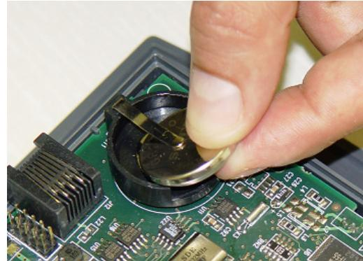
4. Slide the new battery sideways under the clip as shown. The clip must hold the battery securely.
