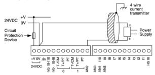
Analog Input wiring, voltage, AN4 and AN5
