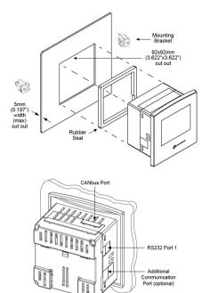
Note: For UL listed module, in order to meet the UL508 standard, panel-mount this device on the flat surface of a Type 1 enclosure.
