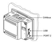
Note: For UL listed module, in order to meet the UL508 standard, panel-mount this device on the flat surface of a Type 1 enclosure.
